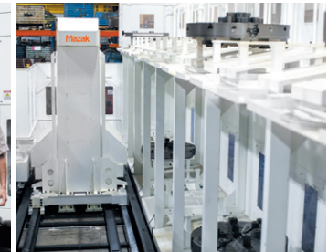
Automation system PALLETECH which enables unmanned operations at night
